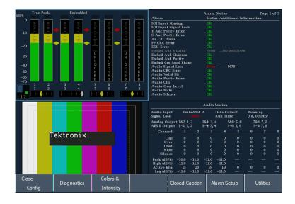
The audio monitor can also display one tile at a time. To select a display to be shown in full-screen mode, touch the tile so that it is highlighted in blue and then press the **DISPLAY** button.
